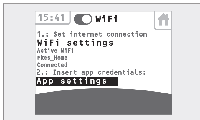
Fig. 3.34 Touch control panel – Wi-Fi receiver switched on
