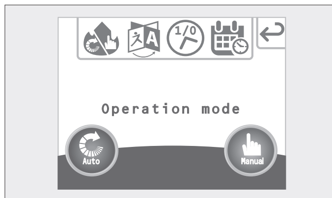
Fig. 3.20 Touch control panel – Operating mode
