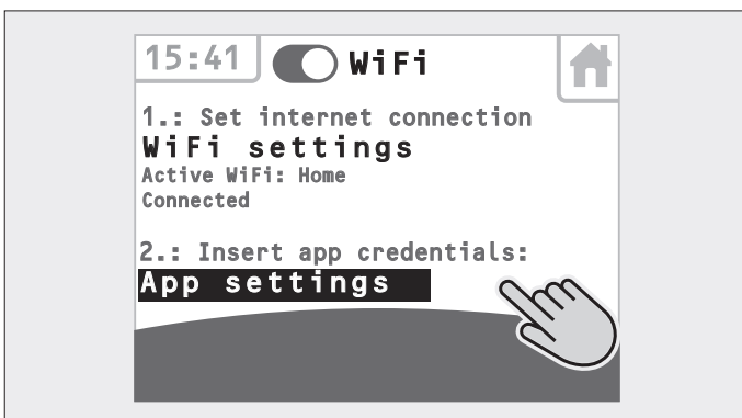
Fig. 3.45 Select app settings for existing Wi-Fi connection
