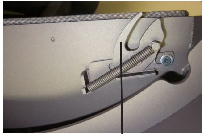
Locking hook in OPEN position
